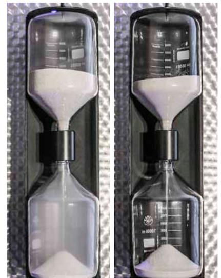
Dorfner apparatus for demonstrating the dust formation characteristics of quartz sand products: (left) standard products and (right) low-dust Dorsicoat brand filler.
